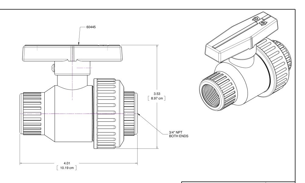
MATERIAL - POLYPROPYLENE WITH TEFLON SEATS EPDM O-RINGS
